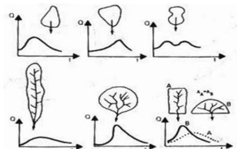
Figure 2. Watershed Hydrograph Form (Strahler, 1957)
