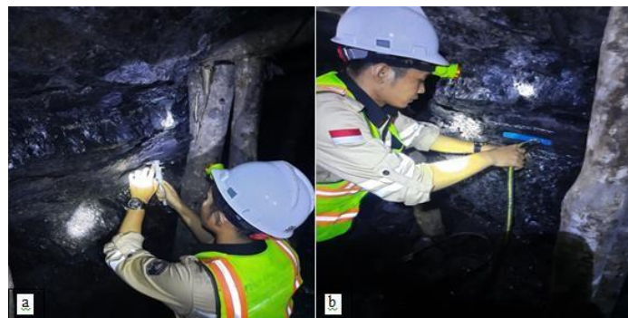
Figure 5. In-situ stress measurement using Flat-jack a) Determination of reference point; and b) Insertion of the plate into the hole that was made.
